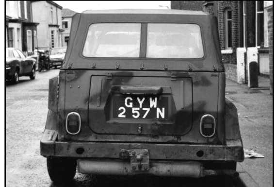
LEFT: This rear window was modified for support and to create a split window effect. Note the elongated muffler, as this one has a Type 4 engine. RIGHT: This one is a right hand drive 182.
