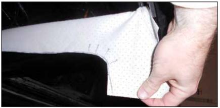
\* **Tip:** Check the instructions on the adhesive. We found applying contact adhesive to the roof, window lip and fabric worked best if we waited for the glue to become tacky. Keep in mind that the glue will remain tacky for up to 30 minutes – take your time to get it right.
