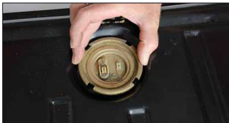
14. Sending unit cap brackets should run up & down
