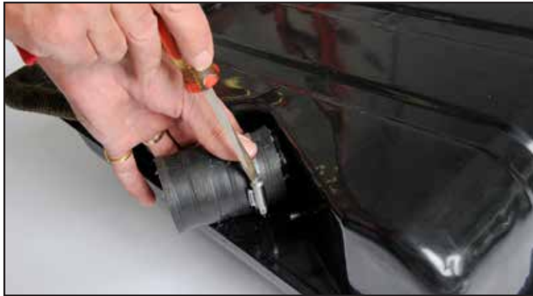
10. Connect new filler neck hose and clamps to new tank
