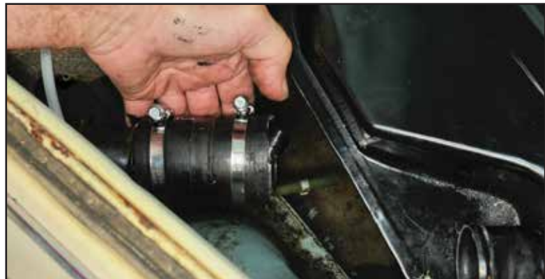
18. Slide new clamps onto filler neck hose. You won't be able to get them on when the tank is installed
