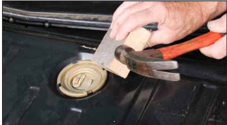
7. Loosen cap on fuel sending unit
