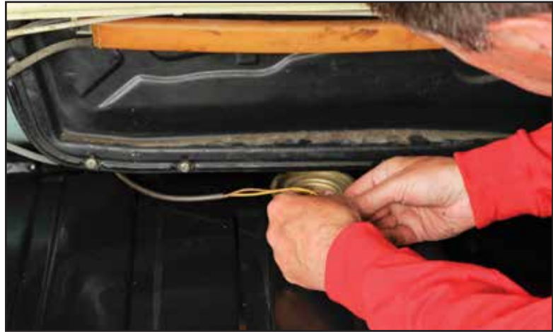
22. Reattach sending unit wires (colored wire head goes on the passenger side bracket)
