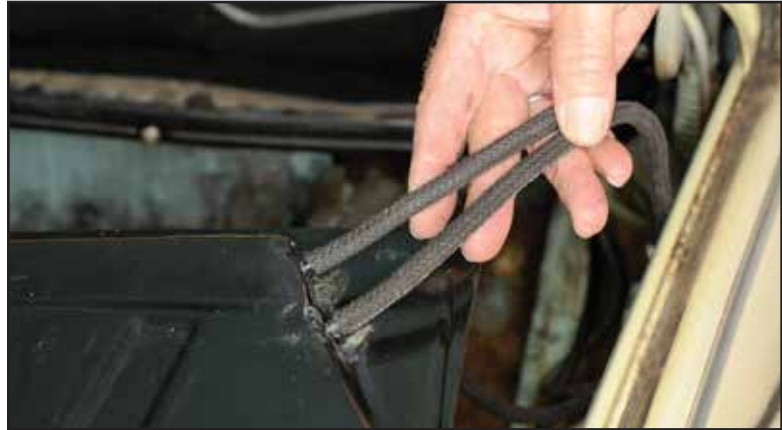
16. Install new breather hoses and attach to new fuel tank
