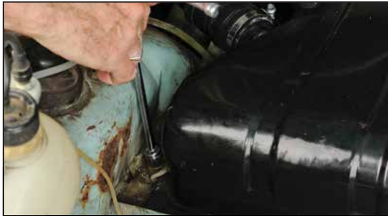
23. Add retaining clamps and tighten
