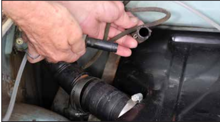
4. Disconnect the Vacuum Hose
