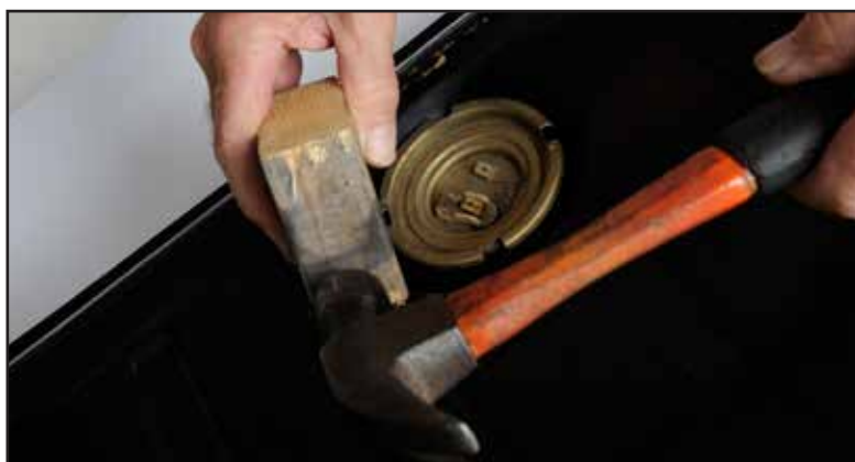
13. Secure the sending unit in place
