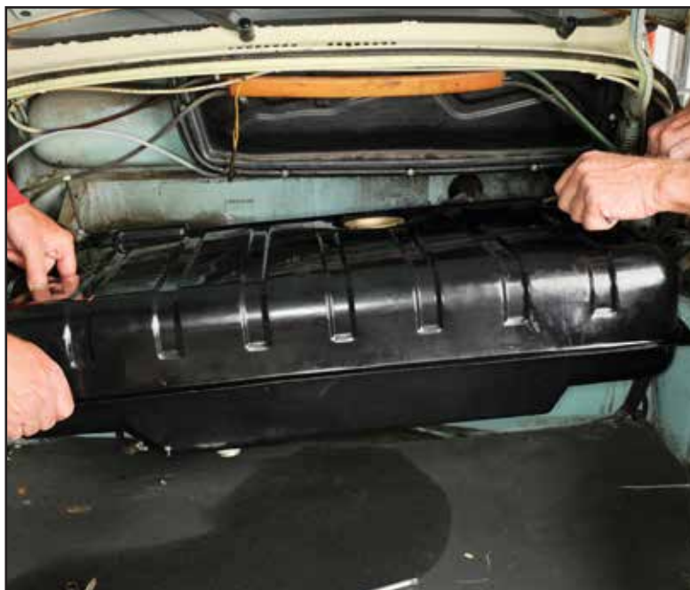
19. Lift & position tank in place
