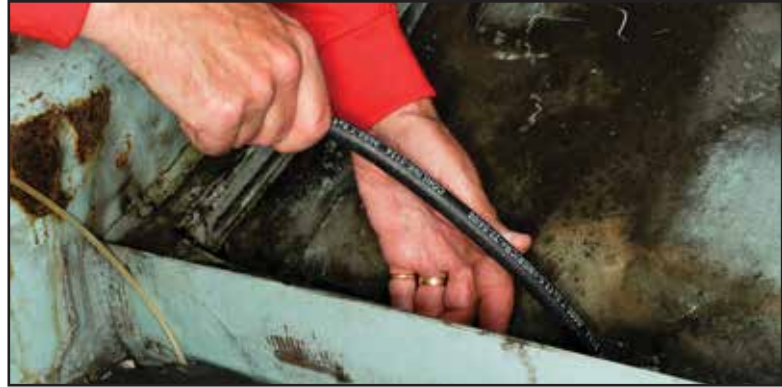
15. Install a new fuel line hose
