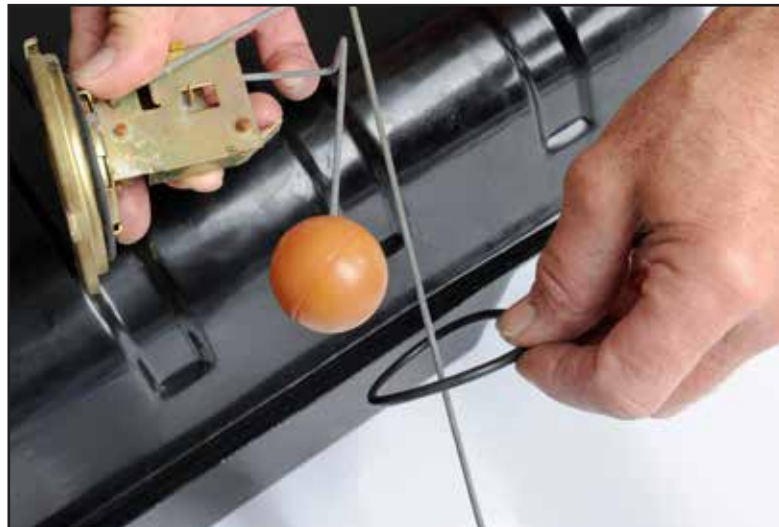
12. Add a new seal to the fuel sending unit (When placing the sending unit into the tank, be sure to feed the sending unit in straight down from the opening for the correct angle.)
