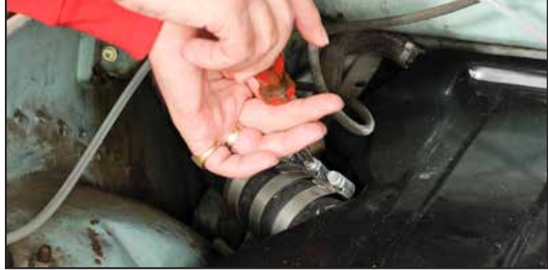
3. Loosen clamps that connect the fuel tank to the filler neck.
