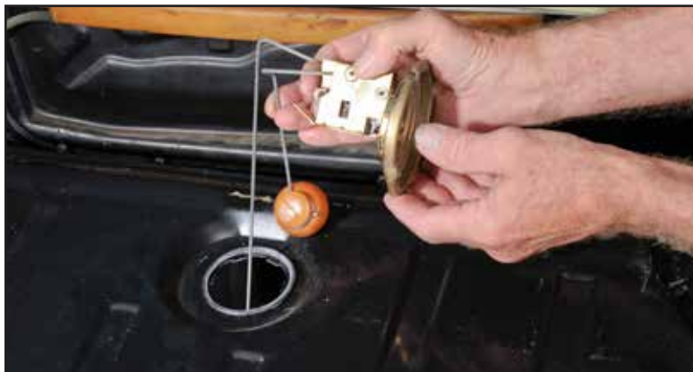
8. Remove fuel sending unit
