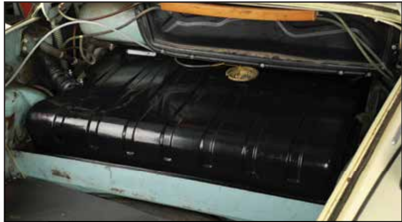
24. After new tank installation
