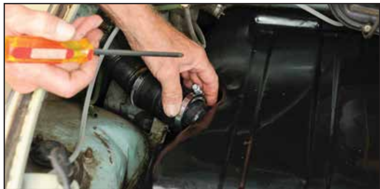
20. Tighten clamps on filler hose. If they are not tight after installation, fuel will leak through and onto your trunk compartment
