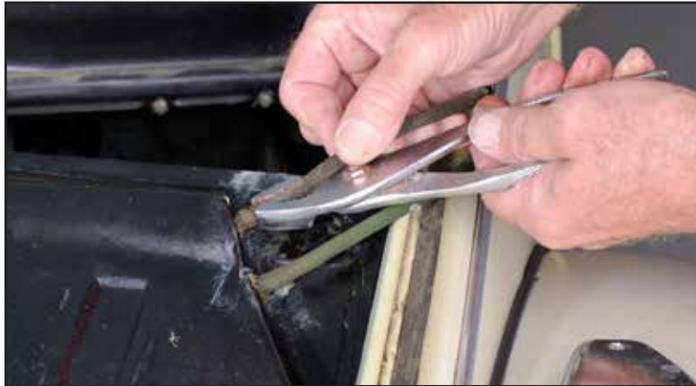
6. Remove breather hoses and filler neck hose (not pictured) from tank
