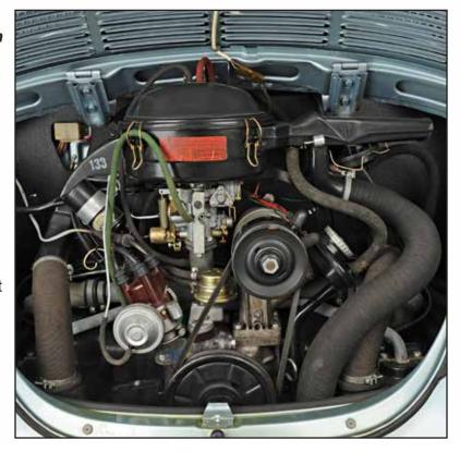
exchangers are only pressed metal around the exhaust header and there are gaps that can allow squirts of exhaust gas to get in around the donut fittings. The male (header) part of those fittings DOES wear as the car ages and it becomes difficult to seal that joint. The end fittings eventually rust out too, but they can be replaced by hammer-in replacement stubs, which also give you a new gas-tight fitting into the muffler.
