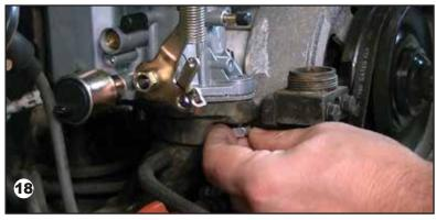
21. Remove the protective covering on the end of the solenoid then reattach the wire coil.
