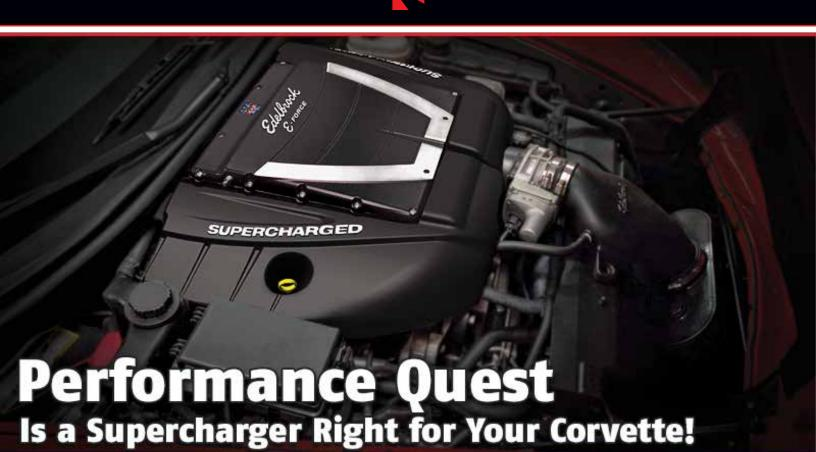
A supercharger is an air compressor that increases the pressure or density of air supplied to an internal combustion engine. This gives each intake cycle of the engine more oxygen, letting it burn more fuel and do more work, thus increasing power. Power for the supercharger can be provided mechanically by means of a belt, gear, shaft, or chain connected to the engine's crankshaft.
