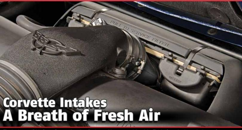
The intake manifold of your Corvette breathes for the car. Yes, you read that right. Think of your intake as the lungs of your Corvette. It takes in oxygen (inhale) for that magical air-fuel mixture that makes movement possible and lets out exhaust (exhale). Mid America Motorworks reviews basic operation of Corvette intakes, as well as the options available to boost performance.
