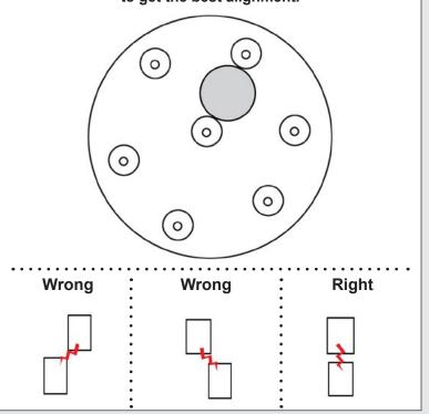
shrouded by the ground electrode faces the center of the combustion chamber, towards the intake valve, as opposed to the wall.
