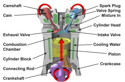
**Stroke 1:** The piston's Intake Valve opens to suck fuel and air into the cylinder.
