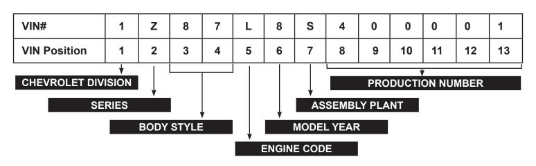
**1978 VINs** included a Corvette first: special identification for Special Edition Models. It was also the first time Chevrolet used a number instead of a letter to identify the engine in the VIN.
