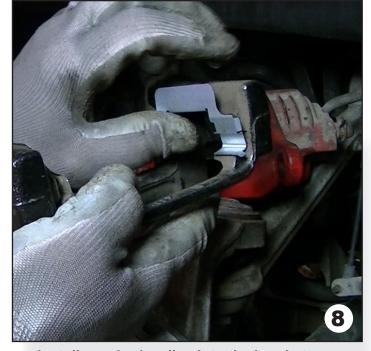
Install new brake clips into the bracket.
