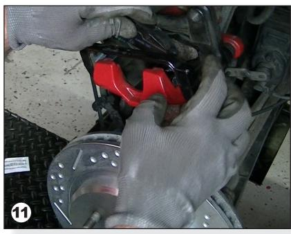
Install new brake pads into the calipers.
