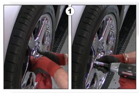
Start by removing the Center Cap of the wheel, then loosen and remove the lug nuts.
