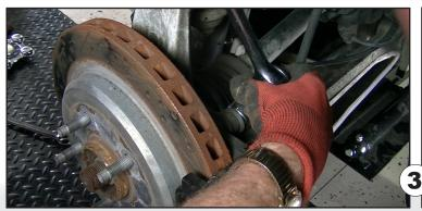
Remove the Caliper Bracket Bolts.
