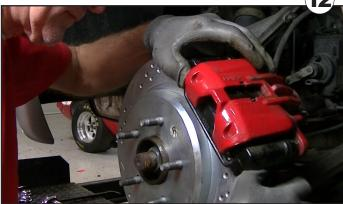
Using a caliper piston compressor tool (104005), compress the piston and set the caliper back into the original position.
