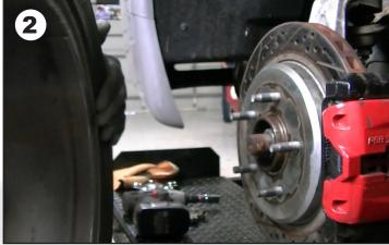
Remove the tire to expose the Brake Caliper.
