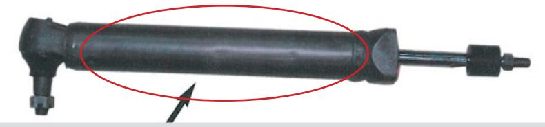
**NOTE:** If your core's cylinder is too severely dented or cracked, these cores are not considered usable and will not be accepted for inspection for a refund. We (and our rebuilders) reserve the right to refuse all of or part(s) of any core sent for inspection if it is deemed unsalvageable
