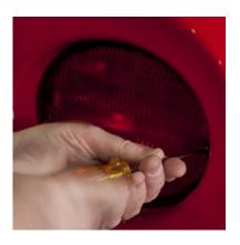
**1.** Remove screws with Torx-15 screwdriver.
