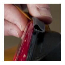
**5.** Starting in the bottom center of the tail light, apply seal to black plastic so rounded edge hangs slightly over the red plastic lens. Trim the end as needed.
