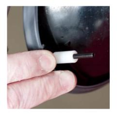
6. Insert Phillips head screws through tail light & place a spacer on the back. Short spacers are for the two outermost screws, long spacers are for 6 innermost screws.
