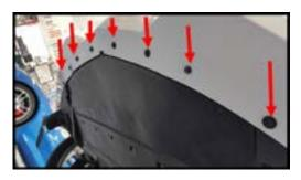
**Step 2:** Some cars will have an oil cooler here. If so, remove the 2 bolts on each end and swing it out of the way. Otherwise, remove the 4 screws that hold the front of the lower radiator shroud. (red arrows). This panel is very flexible, so pull it back and secure with bungie cords as shown. You can see where the LED strip mounts (black arrows).
