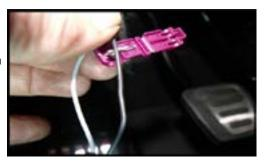
**Step 13:** There is a slot in the back of the connectors. Before you plug them in be sure the wires go above the hood release cables and wiring harness. Connect the red wire to Tan and Black to Black. Make sure lights are now working and be sure lights haven't timed out. Now move to the passenger side.
