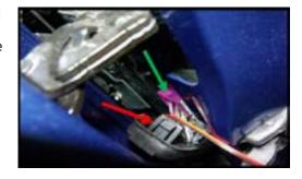
**Step 10:** This is the part that requires a little patience. Its hard to see exactly but you can pass the connectors through on top of the purple block as long as they are done one at a time and the connectors need to be horizontal to fit. You can reach up from inside to grab it once it comes through. Once one is through, gently pull the other one through making sure it is horizontal.
