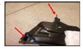
**Step 16:** After all wiring has been completed you need to reinstall the covers on both sides that you released from top of the harness from inside the car. Note: the tab (red arrow) needs to go on top of the wires (green arrow) before pushing it back in to latch it. Be sure not to pinch the wires on top of the tab. The led wires will self seal where the rubber boot seals to the car.
