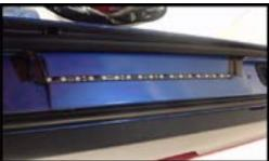
Step 3: Now continue routing the wire behind the weather strip up to this area at the front of the door. There is a pin (green arrow) that holds the W/S in place just below the door strut (red arrow). Route the wire over the top of this pin and push pin back
