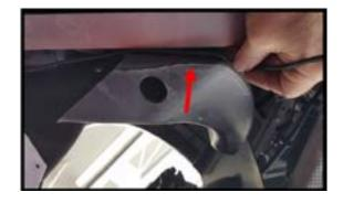
**Step 5:** Line up arrows on the connector and plug it in to the extra lead by the front cove led strip. Tighten the nut.
