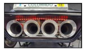
Step 15: Remove the backing from the cable clips before you stick the ends of the led strips. Be sure to prep this area with adhesion promotor. Come back and press the clips in place after a few minutes.
