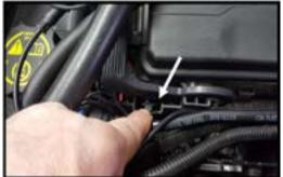
**Step 2:** To gain access to the positive connection release these tabs on each side of the rear of the fuse box while raising the handle. Release the cover over the positive terminal.
