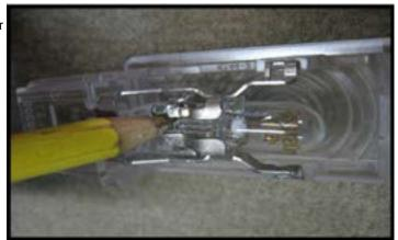
**Step 6.** Install the LED into the light housing. If it doesn't light, remove it turn it 180 degrees and re-install it. Also make sure the lights haven't timed out which they will do after about 15 minutes.
