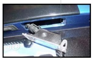
**Step 3.** Remove factory bulb. Be careful, it will be hot! Turn on the lights. Insert LED bulb. If it doesn't light, turn it 180 degrees and re-install. Reverse this procedure to re-install light.
