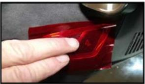
**Step 3.** Work the tint into the edges of the lens around the front side of the lens first. Next move to the rear of the lens behind the button. Lift the tint while working it onto the lens behind and around the button. It tough to get the back of the lens covered without 1 small crease but where its at it doesn't show easily.
