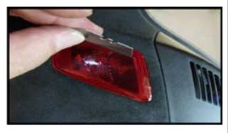
**Step 6.** Remove the tint from the button. If you have to re-do the tint, clean the adhesive residue with wax or grease remover or window cleaner before re applying the tint. Go back and press the tint into the corners and creases one last time.
