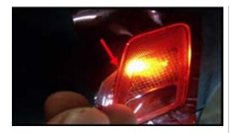
**Step 5.** Trim around the button being very careful on the corners. Use your fingernails to press the tint into the crease.
