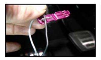
**Step 13.** There is a slot in the back of the connectors. Before you plug them in be sure the wires go above the hood release cables and wiring harness. Connect the red wire to Tan and Black to Black. Make sure lights are now working and be sure lights haven't timed out. Now move to the passenger side.
