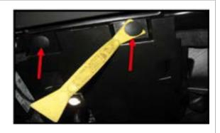
**Step 2.** Remove the factory light by turning it counter clockwise to unlatch it.
