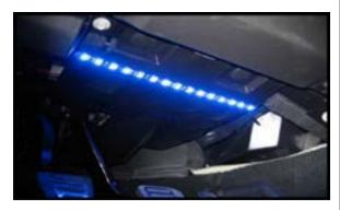
**Step 6.** This shows the best lighting position on the passenger side. Replace the panel, wipe the mounting area with alcohol pads and let dry. Prep with adhesion promoter. Peel the backing and place the strip over the plastic retainers. There will be areas where the strip doesn't contact the panel but will still stay in place. You can now put those factory lights away, you wont need them anymore!
