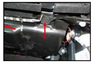
**Step 15.** Remove the factory light housing and complete the wiring for the leds just as you did on the drivers side. After the leds are working, reinstall the factory light and reinstall the above panel. Make sure you pay attention to the plastic pin at the rear. There is a hole in the firewall just above the carpet line. Also make sure you properly insert the heater ducting when pushing it up into place. Then you can push in the retainer pins to hold it in place.
