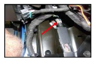
**Step 9.** Look between the 2 door hinges and you will see the cover you just released from inside the car. Pull it back a little to give yourself room to route the wires. Note the purple top of the connector block (green arrow). This is where the wires are passed to the inside of the car. Yes they will fit!
