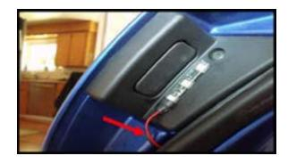
**Step 2.** This shows where the under door strip will be mounted so only apply promotor to this thin area. Use the 2 rivets as a guide as this is how to also line up the strip when installing it. Peel the backing from the strip as you go, lining it up with the rivets at each end. Tape up the exposed wires with strong tape.
