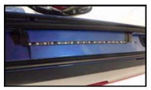
**Step 3.** Now continue routing the wire behind the weather strip up to this area at the front of the door. There is a pin (green arrow) that holds the W/S in place just below the door strut (red arrow). Route the wire over the top of this pin and push the pin back in.
