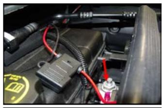
**Step 9.** To gain easier access to the positive connection point, you can raise the large handle out of the way by releasing the locking tab on each side of the fuse box and pulling it up.
