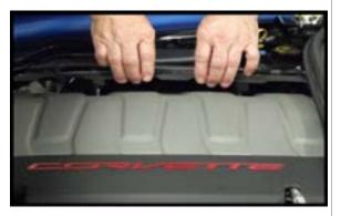
Step 2. This shows the drivers side location of the LED strips. First, wipe down the mounting area with degreaser then alcohol swabs. Next, cut the very top off the adhesion promotor pack. Squeeze the excess fluid back into the packet as you remove the sponge. Re-seal the packet so it wont dry out before you do the other side. Apply a thin coat to the area where the strips mount. Let dry for a 2 minutes. Apply the strips within 1 hr.
