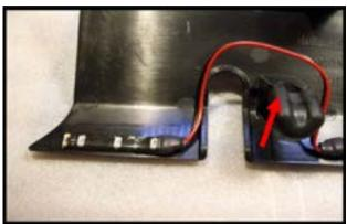
**Step 4.** The backing is easier to remove if you score it with a razor blade as shown. Use caution and don't cut too deep. Use the large picture above to trial fit and mount all the strips. Now use the supplied heat ducting tape to secure the wires.
