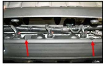
**Step 7.** Connect the coil cover wires together, red to red and black to black. Drop the wires down behind the engine to hide them.
