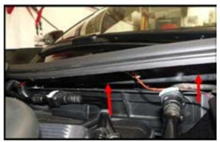
**Step 15.** The long black wire has to be routed up to the ground stud located ahead and below the alternator. Secure the black wire with the provided nut and tighten. Now hide and secure all wires and use the supplied cable ties to secure them. Always re-check wires and strips after a while to be sure they are all secure. You can install 1/4" wire loom over any exposed wires to hide them better.
