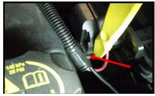
**Step 11.** Remove the 13mm nut and connect the fused red wire. Point the red wire so it follows the factory cable so you can close the cover.
