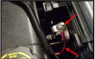
**Step 12.** The red dot shows where the hood bumper hits so do not drill the hole there. Drill a 3/8" hole as shown. Put a towel under this area to catch the filings. Be careful to not drillinto things under this brace. If yours is a Z51 car, be careful of the lines under this bracket.
