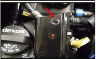
Step 13. Slide the switch through the hole, start the nut then plug the black wire into the bottom before tightening the nut. Hold the top nut with the 7/16" wrench and tighten the bottom nut with the 9/16" wrench. It is a nylock nut so it will be hard to tighten but it won't come loose! The LEDs should now light. Test the switch operation by closing the hood and observing if the lights go off. If not, you can raise the switch by placing a 3/8" washer under the top nut.
