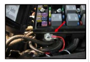
**Step 10.** Below the battery tray (white arrow) along the frame rail there is a ground nut (red arrow). Place the black wire from the control box over this stud and attach with the provided nut.
