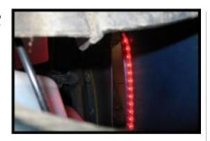
**Step 8.** On the passenger side, Use a coat hangar to find a path down to the cove area (red arrow). Route LEDs down to the cove opening and use the same procedure to mount them as the drivers side. Mount on the inside of the fender facing the cove shield (white arrow). IMPORTANT; Use some very strong tape such as duct tape or gorilla tape to secure the wired end of the strip to the inner fender.
