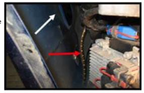
**Step 9.** Open the cover over the positive battery connection at the under hood fuse box. Place red wire from control box over this stud and secure with provided nut. You can also connect it to the battery.
