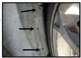
**Step 4.** Using a panel removal tool and a shop rag to protect paint, pry between the panel and fender to unlatch these clips. The one at the top of the fender has a hooked retainer so remove the 2nd and 3rd ones first.
