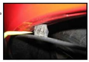
**Step 5.** Shield removed to gain access to cove area. LEDs will drop into this area for installation.
