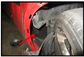
**Step 6.** If removing the cove shields you need to remove these 2 screws from the rear of the fender. Open door, put protective tape around this area to protect the paint. The shield is also held on by 2 adhesives.
