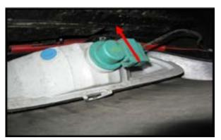
**Step 2:** Remove and unplug the factory bulb. It pulls straight out of its socket.
