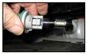
**Step 4:** Line up the tabs on the socket with the notches on the housing and once it is all the way in and seated, turn the socket clockwise to lock it in place. Repeat on other side and your done.
