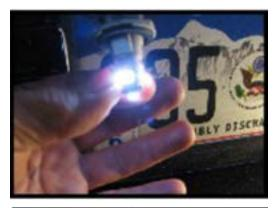
**Step 5.** Re-insert bulb socket into housing and twist 1/4 turn clockwise. Re-attach housing with the 2 torx screws and repeat for the second housing.
