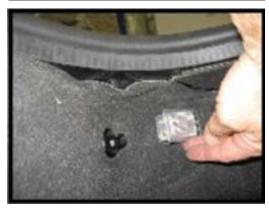
**Step 2.** Remove the bulb sheid by unlatching it from these 2 plastic tabs.
