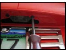
**Step 2.** Remove the light housings, twist the grey socket 1/4 turn counterclockwise to remove it from the housing.
