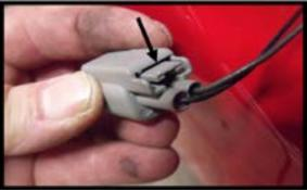
**Step 5:** Feed the led wires through the tailight opening and to the connector you unplugged. Strip back some of the covering on the wires so you can install the connectors.
