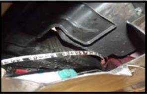
**Step 9:** Wipe the rear edge of the rear fascia where the leds will be mounted with the alcohol pad.
