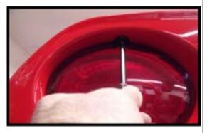
Step 2: Look through the tailight opening and locate the rear side-Marker connector (red arrow). If you can release the latch and disconnect the connector you can wire it without removing the marker light. If not, you will have to remove the marker housing. See next photo.
