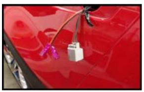
**Step 6:** Place the wire in the metal V and fold the connector closed until it latches. Repeat for both wires.
