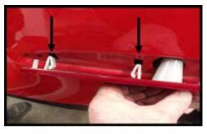
**Step 4:** Release the connector by depressing this tab.
