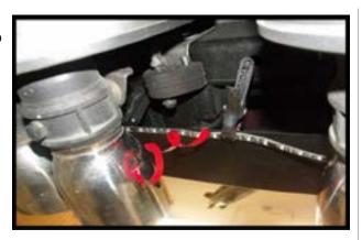
**Step 12:** We prefer to drill a 1/8" hole to secure the wire end of the strip. This keeps this end from possibly dropping down over time. Use the supplied cable ties to secure wiring away from all exhaust pipes.
