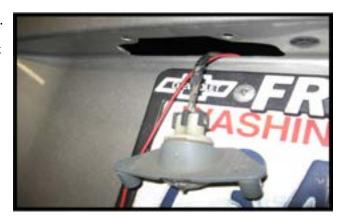
**Step 4:** Strip back some of the tape holding the wires together to give room for the quick taps. Center the wire in the foldable connector and close it together with pliers until it locks in place. Connect the led wires into the back of the connectors. Black to the black wire and red wire to the dark brown wire. Push leads in firmly until they bottom out on the connector as in this picture.
