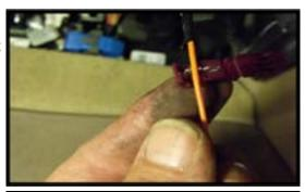
**Step 13.** Now plug in the LED wires to the connectors. Red to orange and black to white as shown. The LED wires just plug into the back of the connectors. Use force to make sure they are tight.
