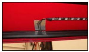
**Step 5.** Remove the rubber plug at the front bottom of the door. Now move to inside the car.
