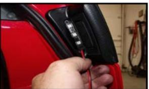
**Step 3.** The weather strip is held by small push in pins. You can release them with a forked tool. Route the wires behind the weather strip down towards the bottom of the door where the leds will be mounted.
