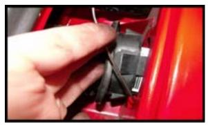
**Step 11.** Un-tape the wires. With one hand feed the wires through the boot, put the other hand in the opening of the inside upper panel you unsnapped and pull the wires through.
