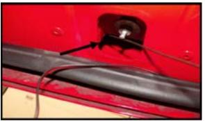
**Step 10.** This shows the feed wire coming out of the boot. Pull the wires through the door.
