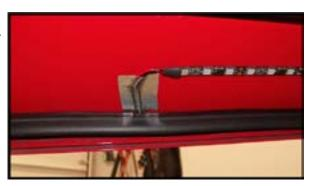
**Step 2:** Using a forked tool you can pry the weather strip retainers out to tuck the wire behind. Route the wire forward toward the rectangular rubber plug located near the front of the door.
