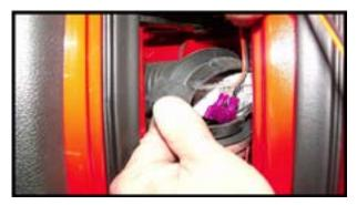
**Step 9:** Locate the factory foot well light wires. They will be orange and white on a C6 and orange and black on a C5. Place 1 wire in each of the metal V of the supplied connectors and snap shut.
