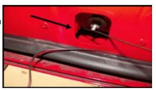
**Step 5:** Open the door and find this rubber plug between the front of the door and the car. Pull the plug loose from the door side so you can put your hand in there to feel for the hangar you are feeding from the bottom (red arrow). Once you have routed the wire hangar through the front of the door, tape the led wires to the wire hangar at the bottom of the door and pull it through the front of the door.
