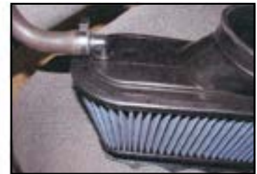
.75" DIAMETER HOLE FOR AIR PUMP
