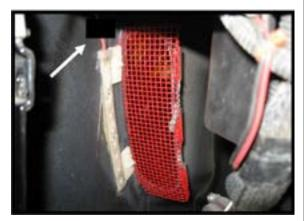
**Step 10:** Now hide the wire under the cowl weather strip. It will help to flatten and tape the wires to the top of the cowl and slip the weather strip over the wires being careful to not damage the wires. You may want to open up the weather strip to make it easier to slip over the wires. You can also tuck the wires behind the battery and engine as long as they don't hit anything that will burn them.
