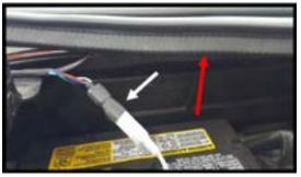
**Step 4:** Next pull the cowl weaterstrip off by pulling it forward. Route the long led wire across the cowl to the drivers side hood latch area.
