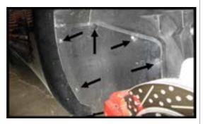
**Step 2:** Remove these 2 x 7mm screws and remove the cove shield Now is a good time to paint the cove shields so they can dry.
