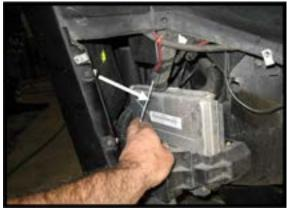
**Step 9:** This car has cove screens over the openings but procedure is the same. Clean the area next to the opening with the supplied alcohol swabs. Peel the backing off the strips and attach to the inside of the fender an inch or two from the opening. **IMPORTANT:** Secure the wires to the fender near the wired end of the strip with some duct tape to keep it from pulling the strip off (White arrow).
