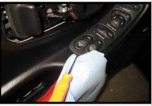
**Step 2.** This shows the passenger side leds after they have been turned 1/8 turn into position. Top LED in the 6 oclock position and the bottom one in the 9 o clock position. Plug the switch in and test the LEDs. Hook the bottom of the switch into the door panel and snap switch back into place.
