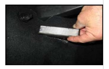
**Step 2.** Turn the bulb socket 1/4 turn counterclockwise to remove it. Pull the factory bulb out and insert the led. Replace the socket and lock it in place. If the led doesn't light remove the socket and turn it 180 degrees and re-insert it. It should now light. The lights will time out after about 15 minutes so keep that in mind if it doesn't light. Push the housing back into the carpet and repeat procedure on the other side.
