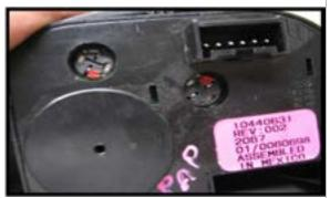
**Step 3.** Using your thumb, press the LEDs into place firmly. Using a flat bladed screwdriver that fits the slot well, twist clockwise 1/8 of a turn until it locks into place. Using the same procedure as on the hatch switch, install the LEDs and twist them into place. Turn on the lights and plug the panel in to test. If they don't light, remove the LED, turn it 180 degrees re-install.
