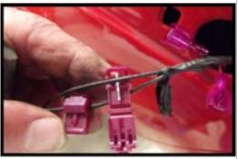
Step 3. This is the area where the LED bar will mount on the rear fascia between the exhaust pipes. Temporarily place the bar here and route the wires up toward the side markers making sure the wires will reach the marker lights once plugged in.
