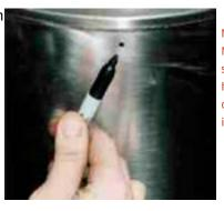
NOTE: IMPORTANT – Make sure that the small drain or weep hole in muffler faces down when muffler is installed
