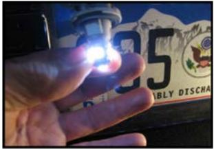
**Step 4:** Turn on the lights. Plug in the led bulb. If it doesn't light, turn it 180 degrees and re-insert.
