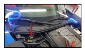
**Step 2:** To gain access to the positive connection release these tabs on each side of the rear of the fuse box while raising the handle. Release the cover over the positive terminal.
