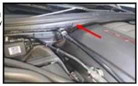
**Step 11:** There are 2 leads on the harness near the control box. One is for the hood vent strip and one for the grill strip if used.
