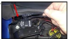
**Step 8:** This shows the LED strip and extra lead inside the fender cove. The extra lead is to connect the rear fascia kit if you are installing it. Use bungie cords to keep fender shield pulled back.
