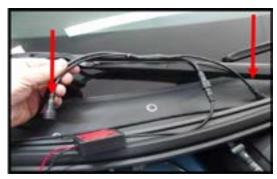
**Step 12:** Now you can mount the hood vent strip. Wipe the mounting area with the supplied alcohol pads. Apply the adhesion promotor to the edge of the ducting. Position the strip as shown. Center the strip on the ducting so the wire comes out as shown in the next picture. Be sure to work the strip into the center and corners as this is the most likely place for it to want to pull off. Keep working it until it fits the corners well.
