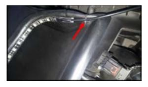
**Step 15:** Route the wire along this tubing toward the connectors on the control box. Secure with wire ties.
