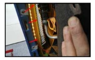
**Step 13:** Lay out the rear kit with the connection lead on the passenger side. Lay the center exhaust section on top of the tailpipes and route the side led strips behind the fascia and out towards the tailight openings hanging the short led strip out of the tailight opening. Place a light behind the lower rear vent so you can see where to route the leds.
