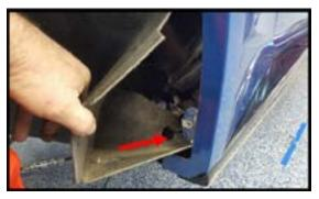
**Step 7:** Route the wire behind the brake scoop up towards the frame.
