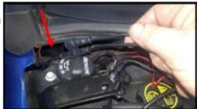
**Step 9:** This shows the led strip and extra lead inside the fender cove. The extra lead is to connect the rear fascia kit if you are installing it. Use bungie cords to keep fender shield pulled back.
