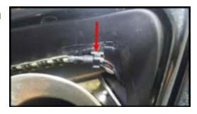
**Step 16:** This is looking down through the tailight opening to show where to mount the side led strips. Mount them a couple inches forward of the vents. Wipe with alcohol then apply adhesion promotor sparingly. Center the strips in the openings and peel the backing off to apply. Always tape the cables to the panel to prevent the strips from pulling off. (red arrows). Repeat on both sides.
