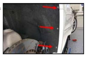
**Step 2:** The inner fender panel is very flexible so you can untuck it from behind the fender then lift the bottom up and out to gain access to the rocker panel area to fish the extension cable from front to rear.
