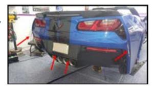
**Step 14:** Wipe the front most edge of the area over the tailpipes with alcohol pads then apply a thin coat of adhesion promotor. Reseal packet so it doesn't dry out. Center the exhaust strip and attach it along the front most edge as shown. Always route cables away from the exhaust.
