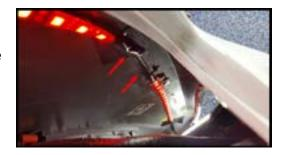
**Step 17:** Now go back and tape down the cables wherever you can. We tape them to the bottom of the rear fascia where the cables go out to the side vents. Wipe the panels first as they will be dirty. Finally bundle the extra cable and tie it up away from the exhaust system.
