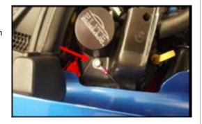
**Step 5:** Turn the wheel out on the side you're working on. Use a pry tool to pop the front splash guards out. There is also a screw underneath if you want to take it all the way off. Repeat on both sides.
