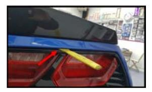
**Step 10:** There are 3 on the top and bottom, 3 on the wide side and 2 on the narrow end. Pull out as you release the tabs.
