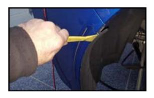
**Step 12:** Looking through the quarter panel you can see the lower rear grills. There are 3 tabs on each side you need to release to remove it. Release the bottom ones then pull out while you release the rest of them. Get the top 2 through the tailight opening.
