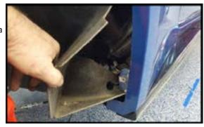
**Step 3:** Looking toward the front of the car in the dark recess you just uncovered there are 2 wads of stuffing that need to be removed. They are stuffed into the rocker panel area to block debris so you may have to reach way in to grab them.
