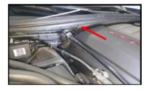
**Step 12:** There are 2 leads on the harness near the control box. One is for the hood vent strip and one for the grill strip if used.
