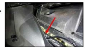
**Step 4:** Cut the very top off the adhesion packet. Squeeze the excess fluid back into the packet as you remove it. Fold the top over and seal to preserve the remaining fluid for use on other kits. Center the strip in the grill opening and mount it to the bar as shown. Tape the wired end down with duct tape.
