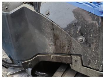
6. The rearward most rear under tray is secured by two push clips (1 per side), four T15 TORX screws (2 per side), and six 7mm bolts (3 per side). Remove the push clips first using a removal tool or flathead screwdriver, followed by the T15 TORX screws, and then the bolts using a 7mm socket and ¼" ratchet. This will free the rearward under tray from the vehicle. Set aside the rearward under tray and fasteners in a protected location.
