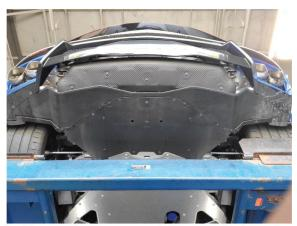
4. The rear bumper cover, two rear under trays, two inner fender liners, and the rear wheels will all need to be removed first in order to allow removal of the bumper cover
