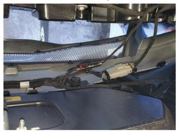
16. (Continued) followed by the two passenger side connectors to free the rear bumper cover from the vehicle. CAREFULLY set aside the factory rear bumper cover in a protected location.
