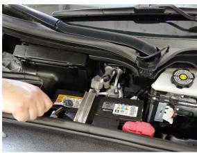
Disconnect the negative battery terminal using a 10mm socket and 3/8" ratchet.
