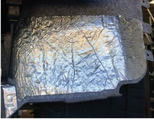
17. Locate the silver factory heat shields that are attached to the wheel well liners. Clean them thoroughly and make sure they are free of dirt, oil and other contaminants.
