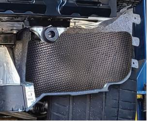
**18.** Test fit the two black shield to each side. Peel back top of release liner and line up along the top of the silver shield and press in place. Once the top is adhered, reach behind the shield and slowly pull backing liner down while pressing the shield in place. Press firmly to make sure shields are competely adhered. The adhesive is very aggressive. Take your time to get original position correct.
