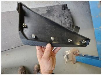
Unclip the two rear splash guard panels from the outside rearmost corners of the inner fender liners. Set aside the panels in a protected Location.
