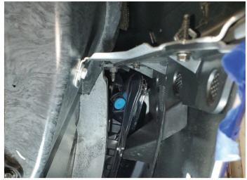
11. The sides of the rear bumper cover are secured to the fender by a 10mm nut and two 7mm bolts on each side. Starting on the driver side, remove the nut first using a 10mm socket and 3/8" ratchet, followed by the two bolts using a 7mm socket and 1/4" ratchet.
