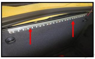
Slide the led bracket over the trunk liner. Center it over the 2 net retainer nuts as shown.
