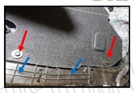
Remove 2 x 7mm screws and pull panel down. The led strip will mount on these 2 ribs (blue arrows)
