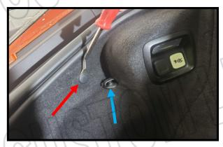
Remove the trunk net. Using the panel tool remove the flat retainer (red arrow). Unscrew the net retainer. (blue arrow).
