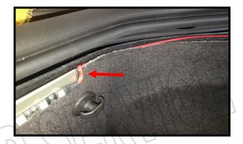
Slide the led bracket over the trunk liner. Center it over the 2 net retainer nuts as shown.
