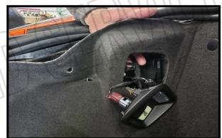
Pull back the trunk liner and push out the retainer clips and remove the light housing.
