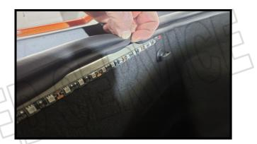
Pull the lip of the weather strip over the exposed portion of the led bar hiding the wire the best you can. Do this around the entire weather strip that you remove. That's it! Enjoy the new lights.
