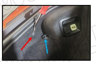
Remove the trunk net. Using the panel tool remove the flat retainer (red arrow). Unscrew the net retainer. ( blue arrow).
