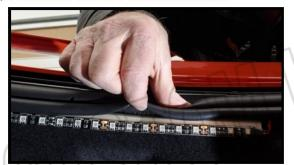
Install the weather strip u channel over the trunk outer liner while pulling the front lip of the weatherstrip out to cover the led channel bracket and inner liner.
