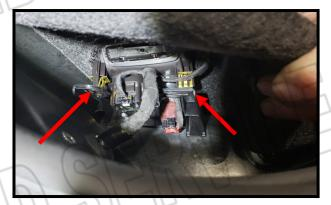
Re-install the light housing by lining up the clips with the bracket openings. Support the bracket from behind while pushing the light housing back In place.
