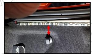
With the led strip with the connector end on the passenger side, slip the channel over the trunk liner aligning the slot on the back of the channel directly above the trunk net retainer. The channel is flexible so you can shape it to match the slight bend in the trunk.
