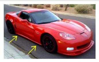
Position the side skirt to line up with the body lines of your Corvette. A second pair of hands to hold the skirt in position will make the install go much smoother. Attach the rear of the side skirt to the splash guard piece with two screws.
