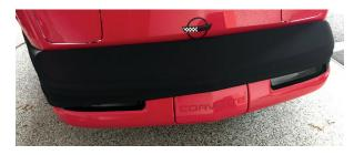
Stretch the mask across the front of the bumper and attach to the other side of the car. (Note: the bottom of the mask can be identified by the label located along the bottom edge of the mask.)
