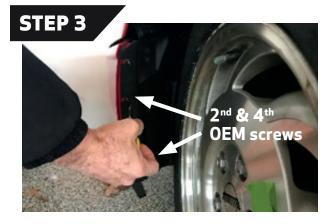
Locate the fender liner mounting screws at the edge of the bumper inside the fender well. Loosen all four screws, this will make it easier to gain access to the two (2) U-clips that you will be removing.
