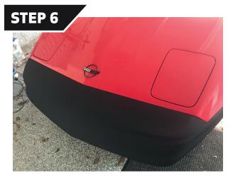
With the hood open, adjust by hand the top of the mask into the hood opening to ensure a clean and complete installation. Close and latch the hood.
