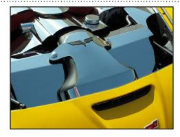
Remove the top of the air tube stud retainer ONLY NOT THE ENTIRE STUD. This will expose a small hole at the top of each stud.
