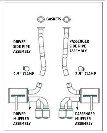
install the driver's side pipe assembly and fasten it at the 2-bolt flange location to the OEM H-pipe using the supplied gaskets and OEM fasteners. Install the passenger's pipe assembly in a similar fashion.
