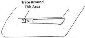
When done tracing, remove the lock knob insert plate from the panel.
