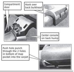
**2.** Remove the console. Lift the back cargo area carpet and push the pointed tabs of the fastening panel through the punched holes as shown.
