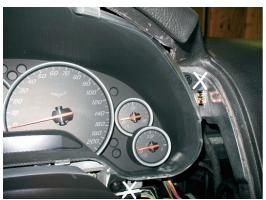
7. Remove the cluster unit from the console. Make sure to clear the console while you pull it out. You might need to life the console a bit to remove.
