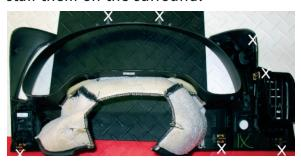
6. Remove the cluster from the pod. The four screws are shown below.
