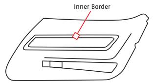
Once aligned, press down on the insert plate with your hands. Press hard enough so the 5- mounting posts on the back of the plate leave indentations in the textured area-on the face of the panel. Remove the insert plate from the panel.
