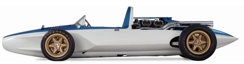
The wheelbase is 96 inches and the car weighs approximately 1600 pounds, ready to run. The foundation is an extremely stiff frame of chromemolybdenum steel tubes welded into a truss-like structure weighing approximately 125 pounds.
