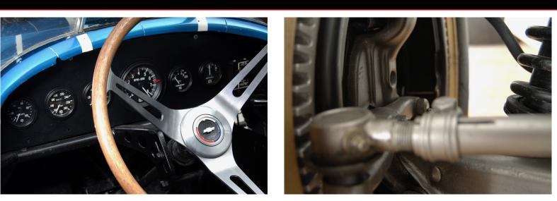
The steering system features a high-efficiency recirculating ball type steering gear of 12:1 ratio. Steering linkage is forward mounted and is of a balanced relay link type. The overall steering ratio is a very fast 13. 5:1 and only 2-1 /4 turns of the steering wheel are required from lock-to-lock.
