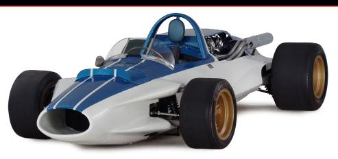
Another fundamental factor in the experimental car's design is the visibility afforded by the body design. The streamlined, abbreviated body encloses the engine, transaxle, engine cooling system, and provides an open cockpit for the driver, from which all four wheels, in contact with the ground, are clearly visible.
