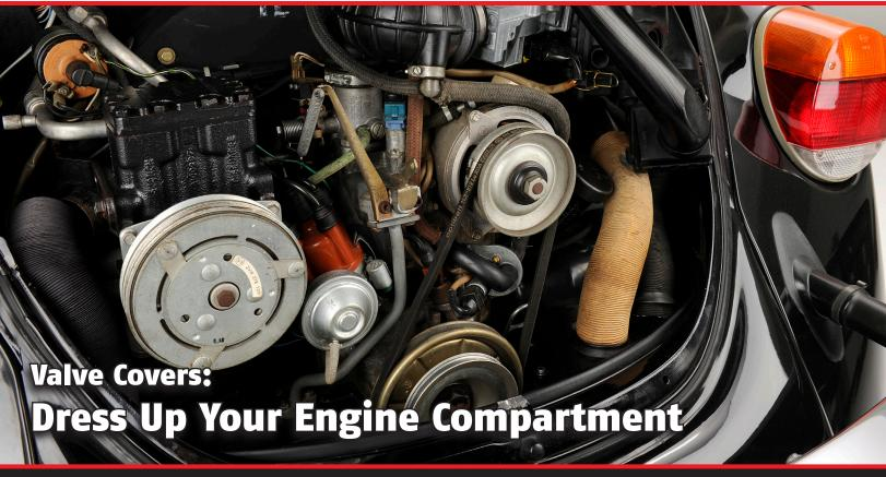
Valve Covers do just as the name suggests – they cover the valve-train components of your Air Cooled VW engine, preventing dirt and debris from entering the system and preventing oil leaks. They are also an inexpensive and simple way to add a custom look to your engine compartment. Mid America Motorworks reviews the different Valve Covers available, along with hardware options, to make your engine compartment take center stage.
